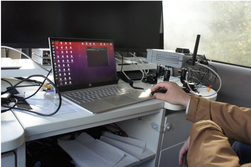
Figure 3 Inside the test vehicle with ground station PC and VINS-RTK enclosure
